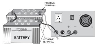
In series connection positive terminal of one battery is connected to the negative of other battery.
