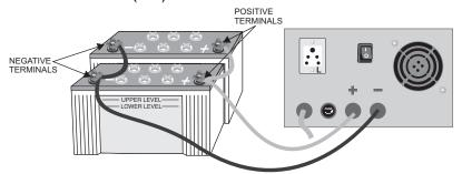
In parallel connection positive terminal of one battery is connected to the positive terminal of other battery & negative to the negative terminal.
